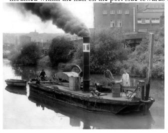
was passed into the boiler flue and up the funnel, giving the boat a distinctive pulsing roar when in motion.
